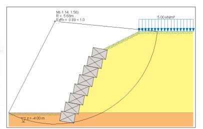
Inclined layered blocks with offsets
